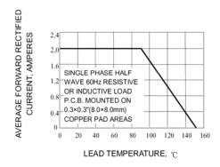
Fig. 1-DERATING CURVE FOR OUTPUT RECTIFIED CURRENT
